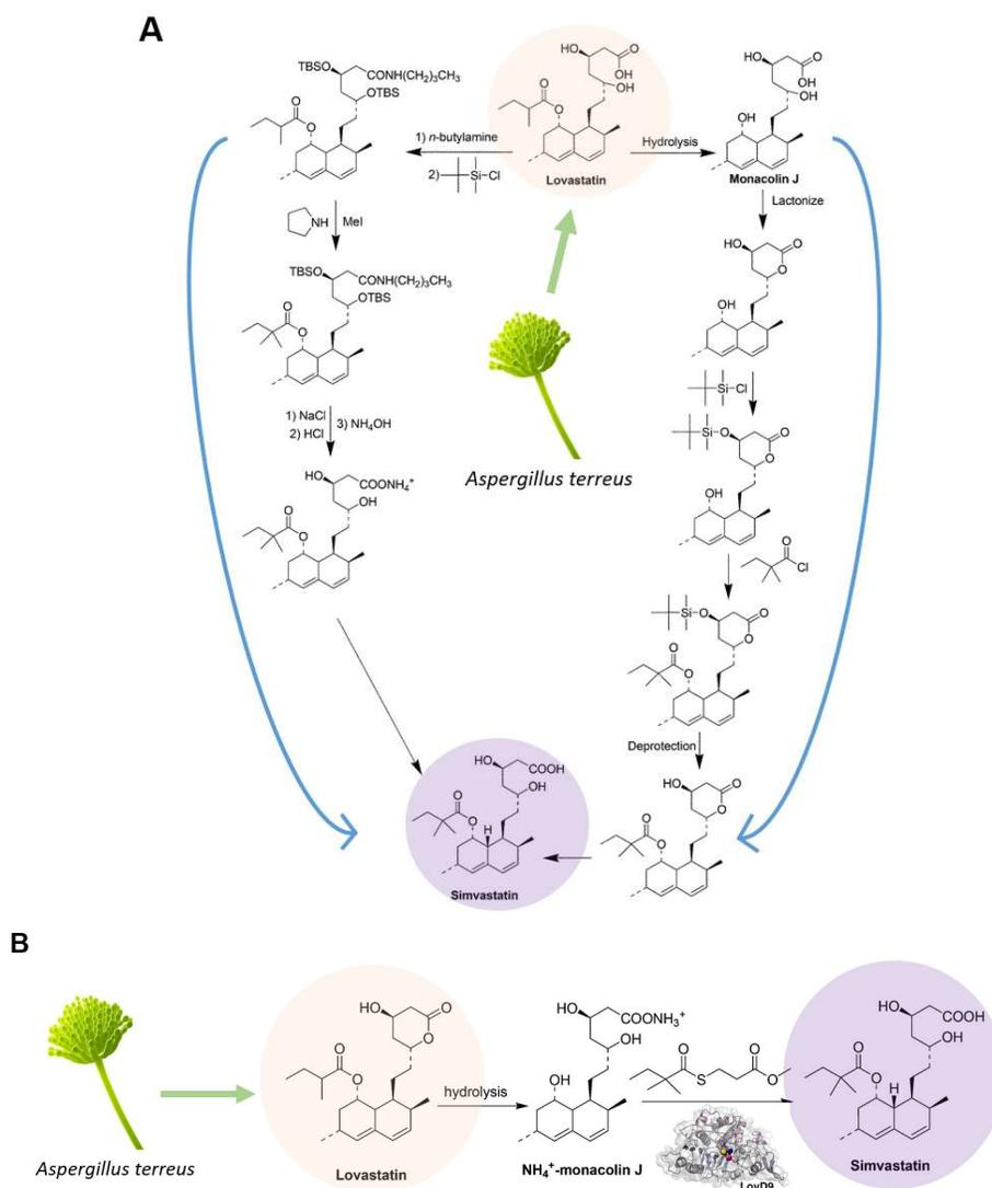
**Figure 1.** Synthetic methods for cholesterol-lowering agent simvastatin. (A) Traditional chemical syntheses. (B) Chemo-enzymatic synthesis with LovD mutants.
