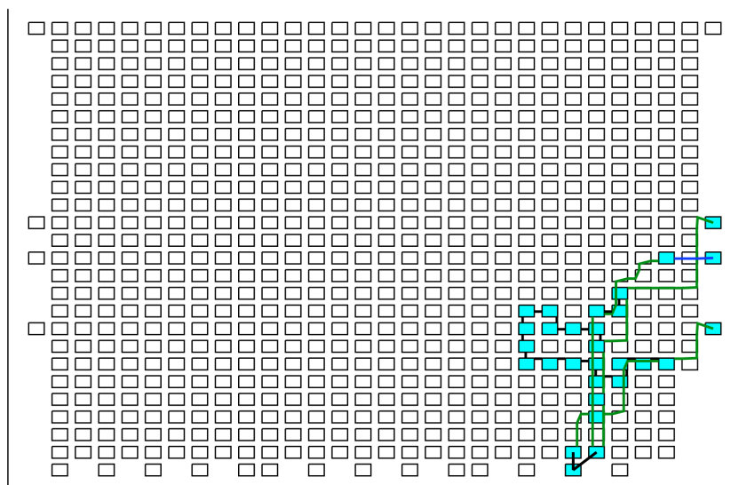
Figure 4.6: The entire optimized decoder application described in Section 4.2.2 is mapped to 25 processors, a single 64 KB memory (on the bottom of the array), and I/O ports on the right edge of the array.
