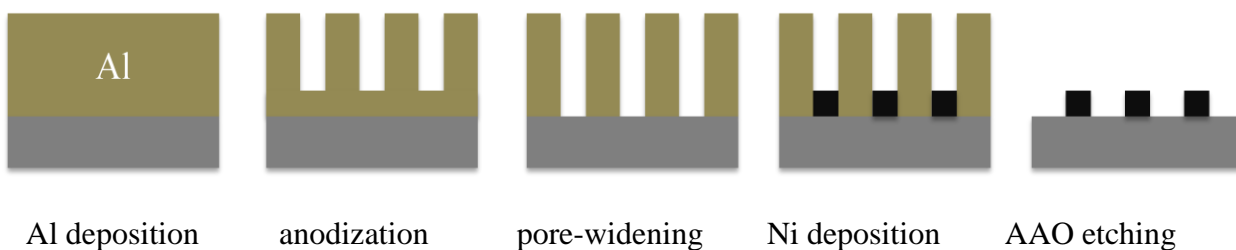
Figure 24. Fabrication of Ni nanodots using AAO template
