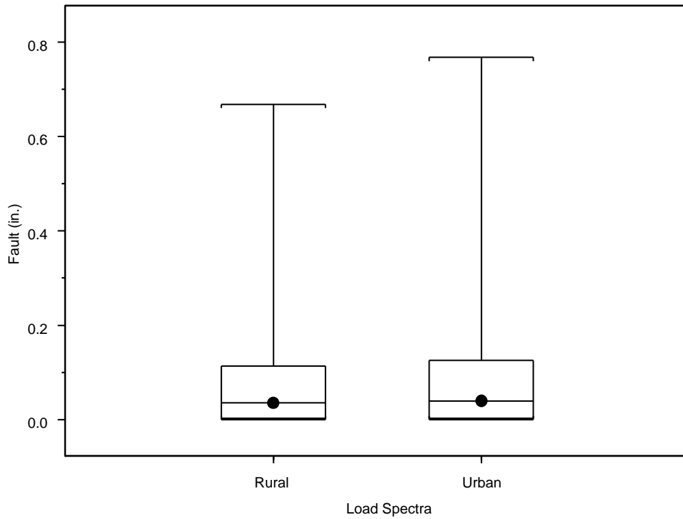
Figure 23. Effect of load spectra on faulting.
