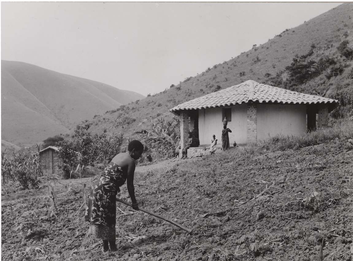
FIGURE 4.7. This round dwelling matches the description of the first kind of house to be built in 1947 as part of a colonial housing program: circular in plan, but constructed with solid materials (bricks, stones, and tiles).
