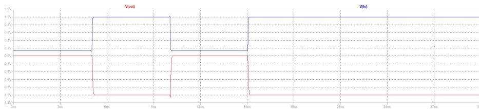
Figure 6.5: Simulated waveform of logic level converter from 1 V to -1 V
