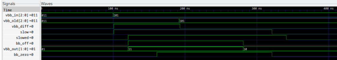
Figure 6.2: Simulated waveform of switching between two non-zero V_{bb} values
