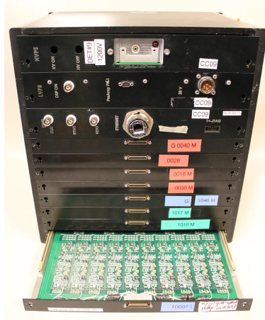
Figure 2.13: A single card cage with one of the analog boards pulled out, showing the 10 pulse shaping circuits. Above the eight analog boards is the DSP board, which handles the trigger logic and relays the data to the flight computer. The next board is the low voltage power supply, which powers both the rest of the card cage and the preamplifiers. The top board is the high voltage power supply which provides 1000 – 1500 V to the detectors.
