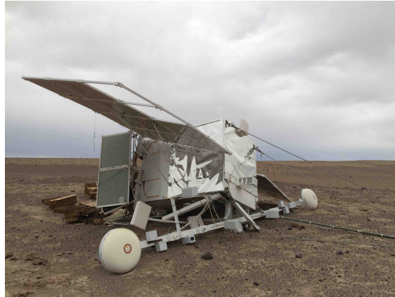
Figure 4.4: A photograph of the COSI payload in at its landing site in Peru, taken by the recovery team. Though the gondola, antenna booms, and solar panels were completely destroyed, the rest of the instrument was unharmed. The GeDs , CsI shields, card cages, and other subsystems have been tested in the lab since the flight and are fully operational.
