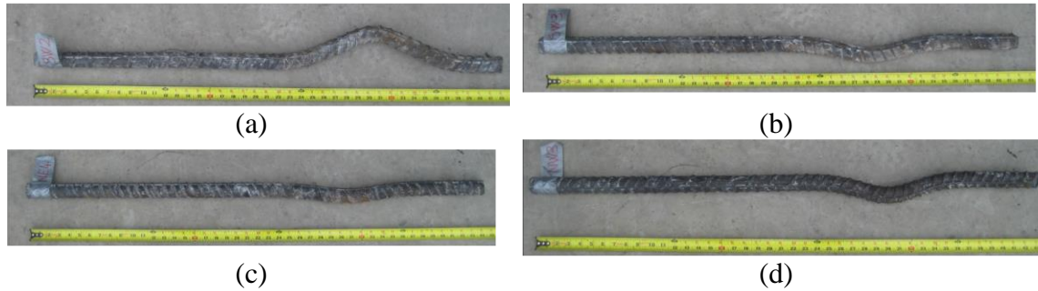
Figure 6.12. Buckled Non-Fractured Reinforcement for Identification of d_{POI} (a) Specimen SW2; (b) Specimen SW3; (c) Specimen NE4; (d) Specimen NW3
