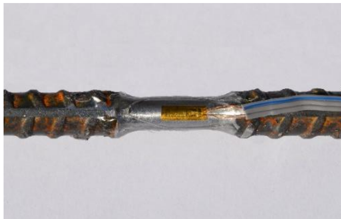
Figure 3.2. Application of Strain Gages to Machined Coupons
