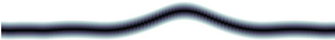
Figure 6.14. Artificial Buckled Shape, d_{POI} = 2.8 d_{bl}
