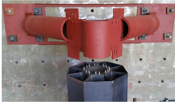
Figure 5.3. View of Bottom Pipe with Heater Terminals and Lateral Bracing System Connected to Strong-Wall
