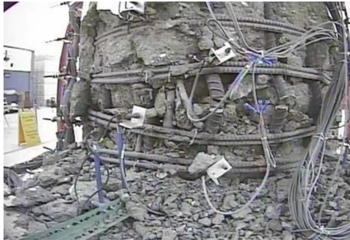
Figure 6.11. Column Base East Face View after EQ10 (Schoettler et al., 2012).
