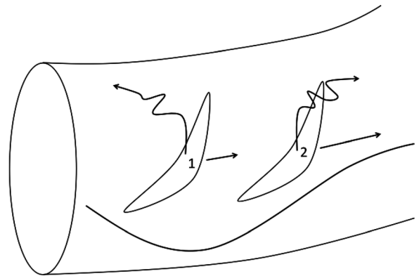
FIG. 6. A cartoon for decorrelation process. 28 Two correlated bananas are decorrelated by (i) turbulent E \times B diffusion and (ii) precession motion at different speeds. The synergy of the processes determines effective lifetime of the correlation.
