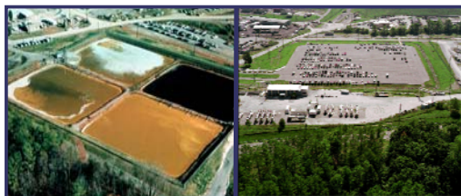
S-3 Waste Ponds. The four unlined S-3 waste collection ponds were constructed in 1951 (left). Effluent waste, consisting primarily of nitric acid, nitrate, metals, and radionuclides (U, Tc), were discharged into the ponds until 1983. The ponds were neutralized and dewatered in 1984 and then capped in 1988. The site is currently covered with asphalt and serves as a parking lot (right). Waste from the ponds seeped into the groundwater and has contaminated the surrounding area, resulting in a site with low pH (3.4-3.6), high U (50 mg L -1 ), and high nitrate (8-12 g L -1 ). (Oak Ridge Field Research Center, 2007).
