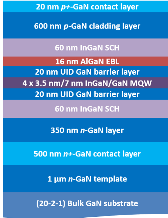
FIG. 3.1. Schematic of the epitaxial structure of the LD on a (20\bar{2}1) substrate. Reproduced with the permission of AIP Publishing 19
