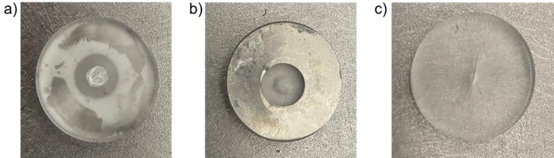
Figure 5.8. The system is currently limited by PMMA substrate that is ablated (a), internally damaged (b), or cracked (c) after 5-20 pulses depending on piece of plexiglass and spacer height.
