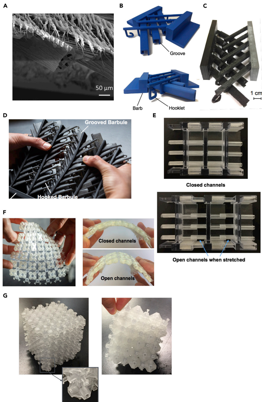
Figure 16. Progression of bioinspired designs based on the attachment mechanism found in the feather vane
