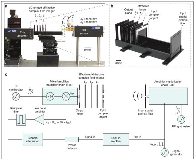
Fig. 7 Experimental set-up for diffractive complex field imagers. a Photograph of the experimental set-up, including a 3D-fabricated diffractive complex field imager. b Photographs of the 3D printed diffractive complex field imager. c Schematic diagram of the continuous-wave terahertz imaging set-up
