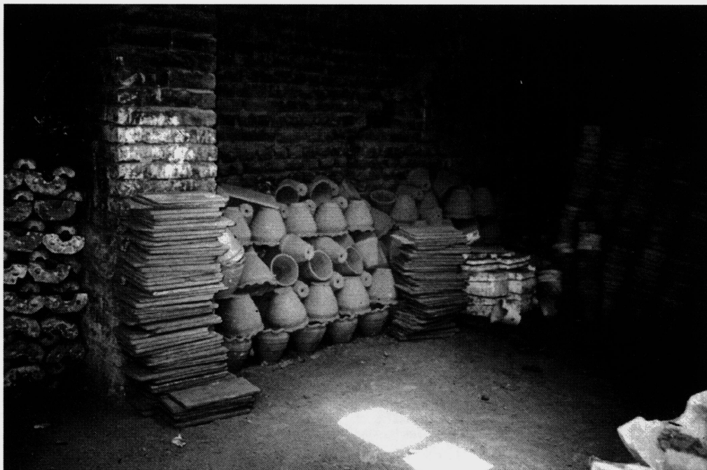
Plate 10.7 Production equipment (note molds to left and boards used to support unfired roof tiles) and completed pots stored against Old Cairo workshop walls.
