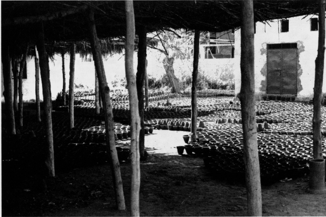
Plate 10.15 Drying sheds at El Qanatar workshop with completed flowerpots drying in the open.
