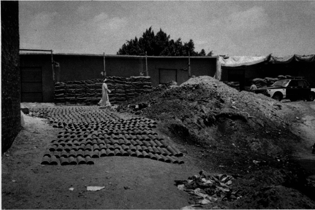
Plate 10.8 View of the front of the Old Cairo workshop looking away from the structure. The car and man in the background are on the unpaved road. To the left are roof tiles drying in the open. To the right is a mound of two different types of unprocessed clay: Nile silt to the right and gebel clay to the left. In the right foreground are ash from the pottery kilns and miscellaneous bits of assorted kiln fuel.
