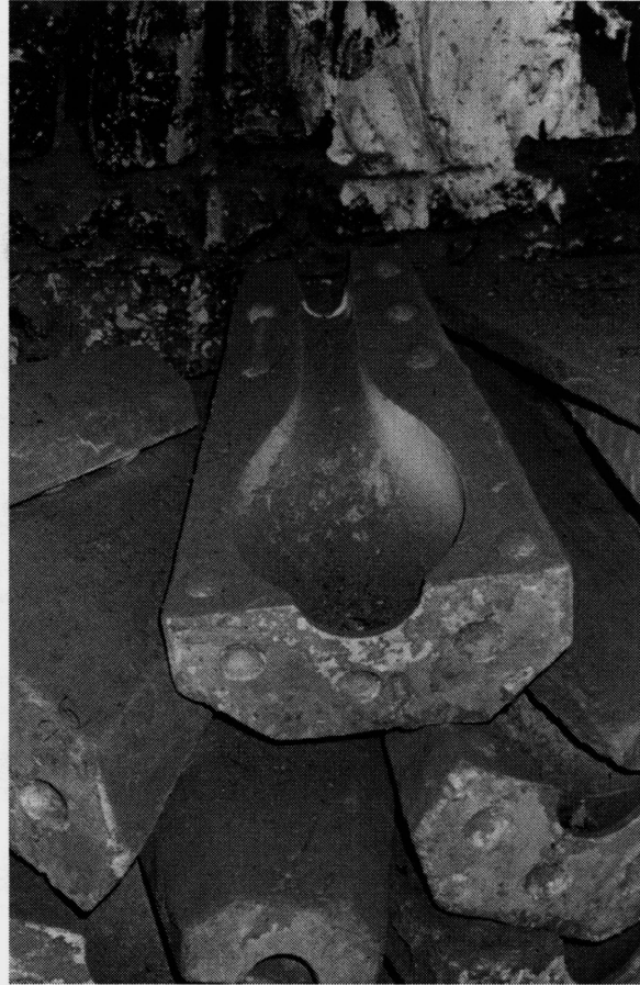
Plate 10.4 Molds for producing candle holders/vases ( šama‘danī ) in the Old Cairo workshop.
