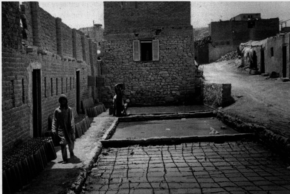
Plate 10.10 The three rectangular settling basins for clay at the Old Cairo workshop. Water remains in the two rear basins but has evaporated almost completely from the basin in the foreground, which is the same basin that appears in the foreground of plate 10.9. Note the two entrances to the workshop to the left and the completed roof tiles stacked against the exterior workshop walls. The girls are two of the young assistants employed at the workshop.
