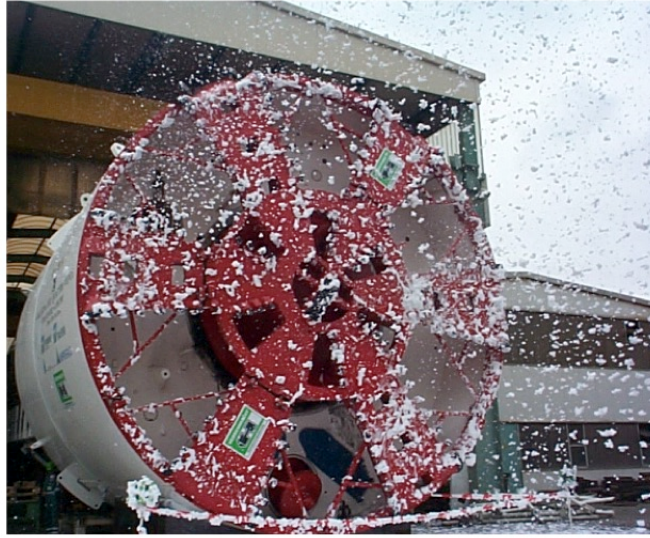
Figure 1.12: TBM testing the foam injection ports on the surface.
