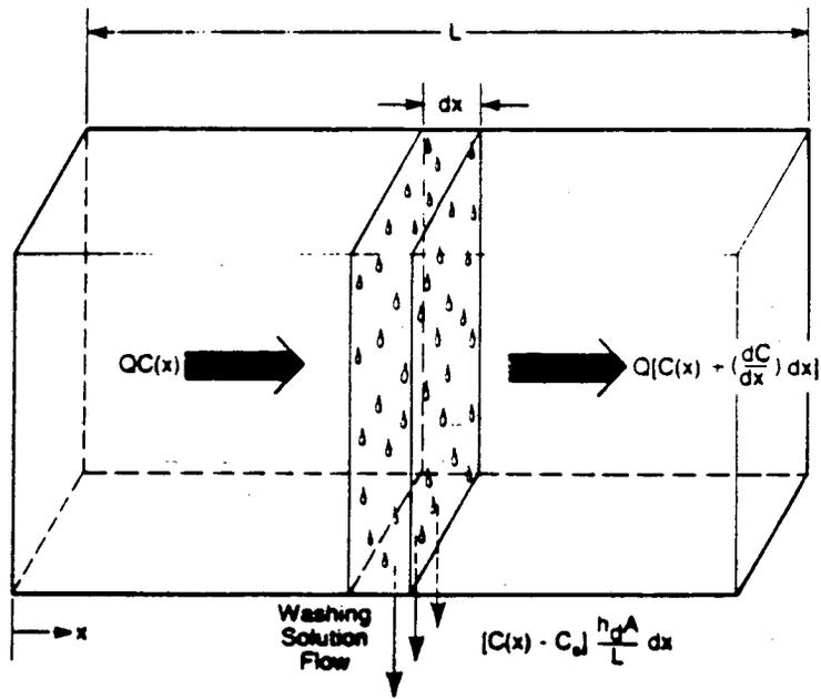
Figure 1. Schematic diagram of control volume employed for derivation of the air washer model. Nomenclature is presented in the text.
