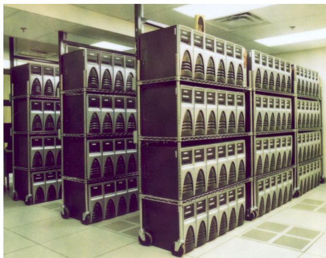
Figure 21.1: Kibbutz100: A 1.1 Teraflops Computer Designed for in Silico Screening and Multiple Molecular Dynamics Simulations. Source: Clinical Pharmacology & Therapeutics.
