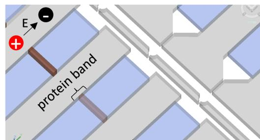
Figure 5.3: Device combines hydrodynamic trapping and electrical lysis for single-cell protein electrophoresis.
