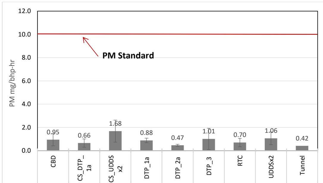
**Figure 8** PM emission factors (g/bhp-hr)
