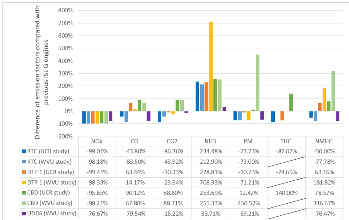
**Figure 12** Difference of emission factors compared with previous ISL G 8.9 engines
