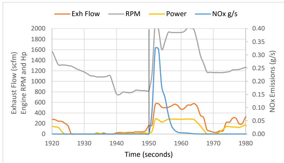
**Figure 3** Real-time NOx emissions compared with Exhaust Flow, Engine RPM and Hp
