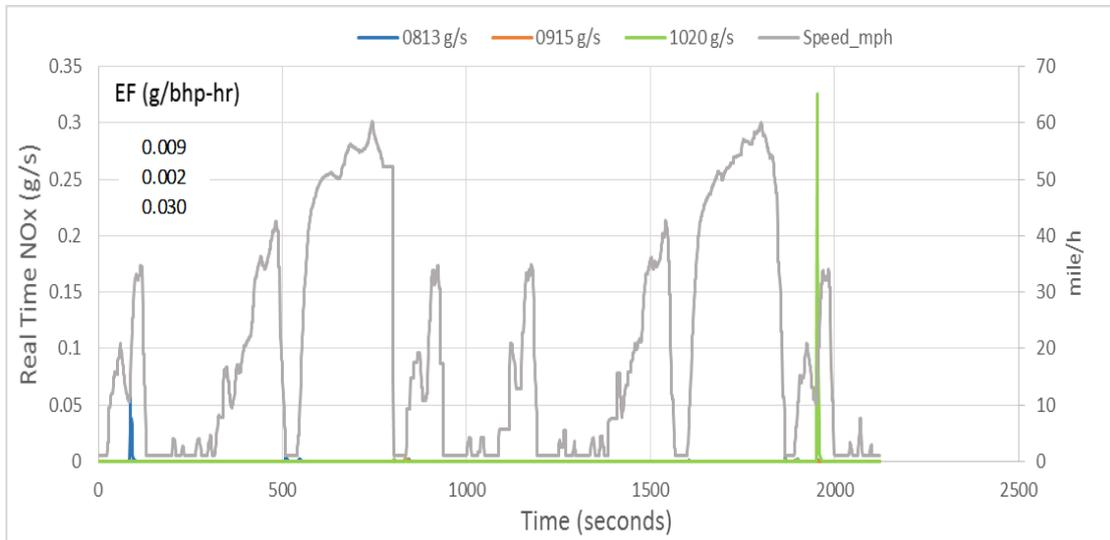
**Figure 2** Real-time NOx emissions of hot UDDS cycles
