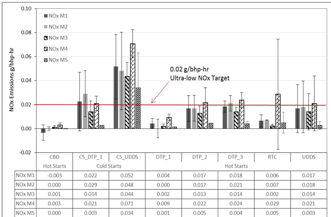
**Figure 1** Measured NOx emissions of 5 methods for the various test cycles
