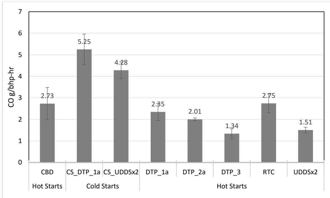
**Figure 6** CO emission factors (g/bhp-hr)
