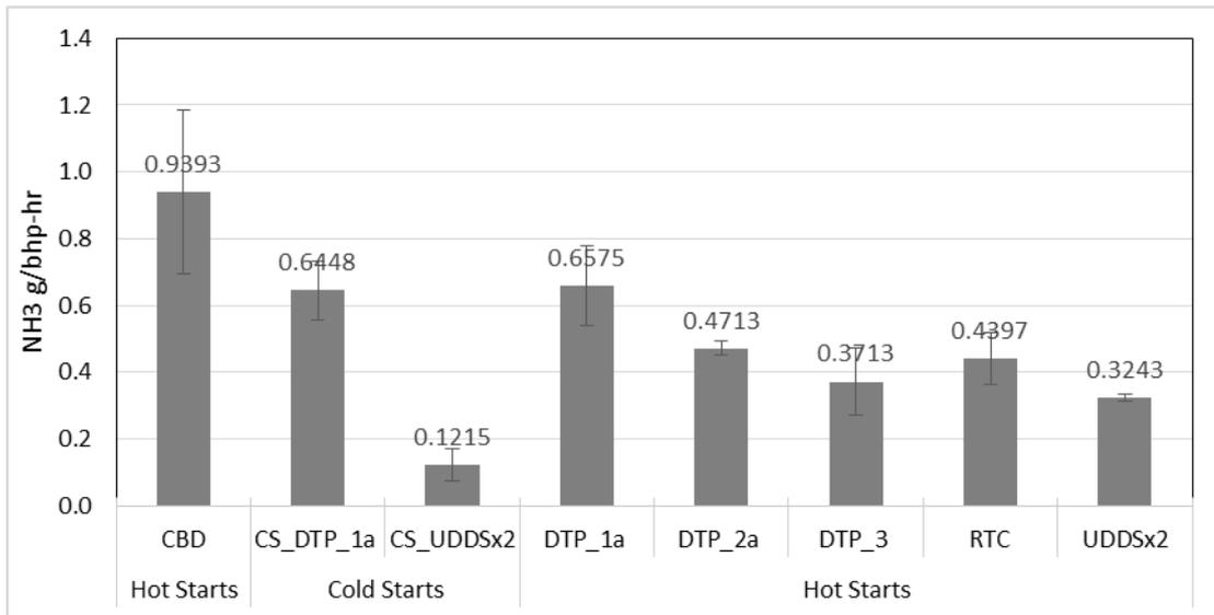
**Figure 7** NH<sub>3</sub> emission factors (g/bhp-hr)
