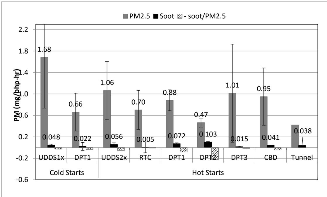
**Figure 9** soot emission factors (g/bhp-hr)
