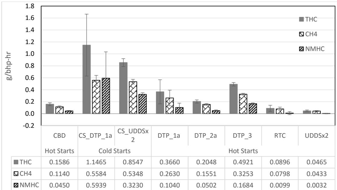
**Figure 5** Hydrocarbon emission factors (g/bhp-hr)
