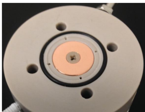
Figure 2. Photograph of working electrode chamber.
