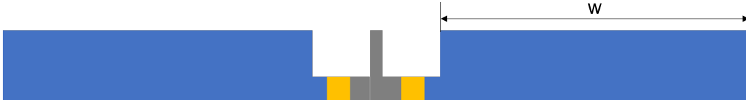
Figure 3.9: Cross section of thermal phase shifter
