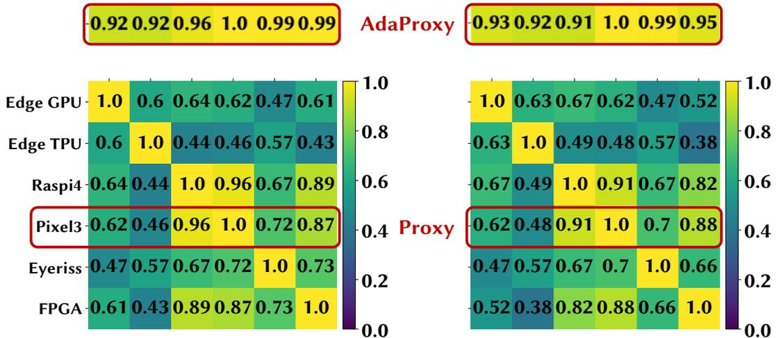
Figure 3.24: SRCC for various devices in the NAS-Bench-201 search space on CIFAR-100 (left) and ImageNet16-120 (right) datasets. Pixel3 is our proxy device. SRCC values boosted with AdaProxy are highlighted.
