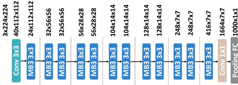
Figure 3.2: An example architecture in the MobileNet-V2 search space, which achieves 70.2% accuracy on ImageNet and 71ms average inference latency on S5e. The text “ $Z_1 \times Z_2 \times Z_3$ ” the input size for each layer.
