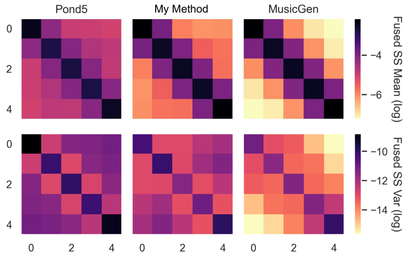
Figure 4.4. The mean (top row) and the variance (bottom row) of the fused self-similarity (SS) matrices are estimated with 100 samples from Pond5, generated by my method, and by MusicGen. The SS matrices are downsampled to 5 \times 5 . The results show that, compared to MusicGen, the samples from my method are more similar to the Pond5 samples in similarity of the parts at long temporal distances.
