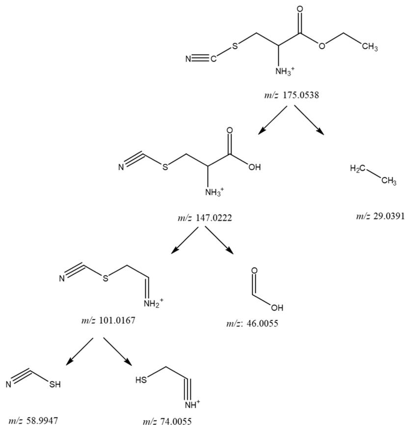
**Figure 3.** Mass spectral fragmentation of cyano-S-ethyl-O-cysteine (CNCysEt). Mass errors are 1.29 mg kg<sup>-1</sup> for C<sub>63</sub>H<sub>11</sub>N<sub>2</sub>O<sub>2</sub>S, -0.51 mg kg<sup>-1</sup> for C<sub>4</sub>H<sub>7</sub>N<sub>2</sub>O<sub>2</sub>S, -0.76 mg kg<sup>-1</sup> for C<sub>3</sub>H<sub>5</sub>N<sub>2</sub>S, -4.09 mg kg<sup>-1</sup> for C<sub>2</sub>H<sub>4</sub>NS, and -5.26 mg kg<sup>-1</sup> for CHNS.
