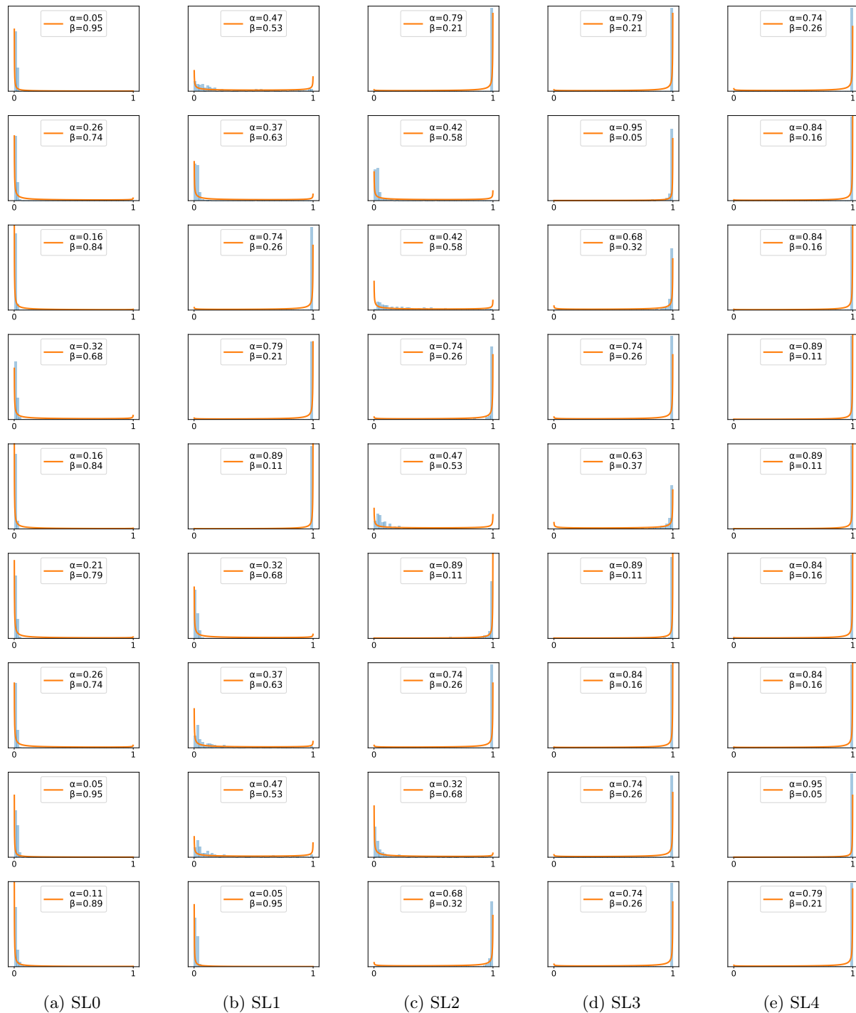
Figure B.2: Histograms showing the spread of trained (with \rho = 0.2 ) NN models' predictions on a selected numbers of data examples from the chiller dataset, and a fitted beta distribution \mathcal{B}(\alpha, \beta) for each example.
