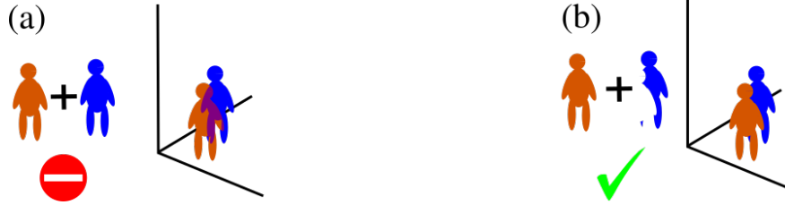
Figure 7.10: Segmentation masks can improve mutual-exclusion constraints. We propose extended mutual-exclusion constraints which enforce this rule: two detections can overlap only if one is occluded . Therefore, two trackers cannot claim two overlapping fully-visible detections, as shown in (a). But in (b), the blue mask was predicted as partially occluded. In this case, the blue and orange detections can be in close proximity and still both be correct.
