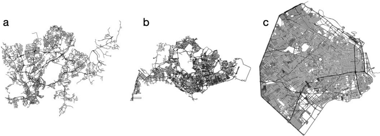
Figure 1. Street networks with (a) small average degree (Helsinki \bar{k} = 2.35 ), (b) typical value (Singapore \bar{k} = 3.0 ), and (c) a large value (Buenos Aires \bar{k} = 3.55 ). The overall organization of street networks is diverse, reflecting a wide range of patterns and structures depending on urban planning, geography, and cultural factors (see the Supp. Info. for details about the degree k calculation).
