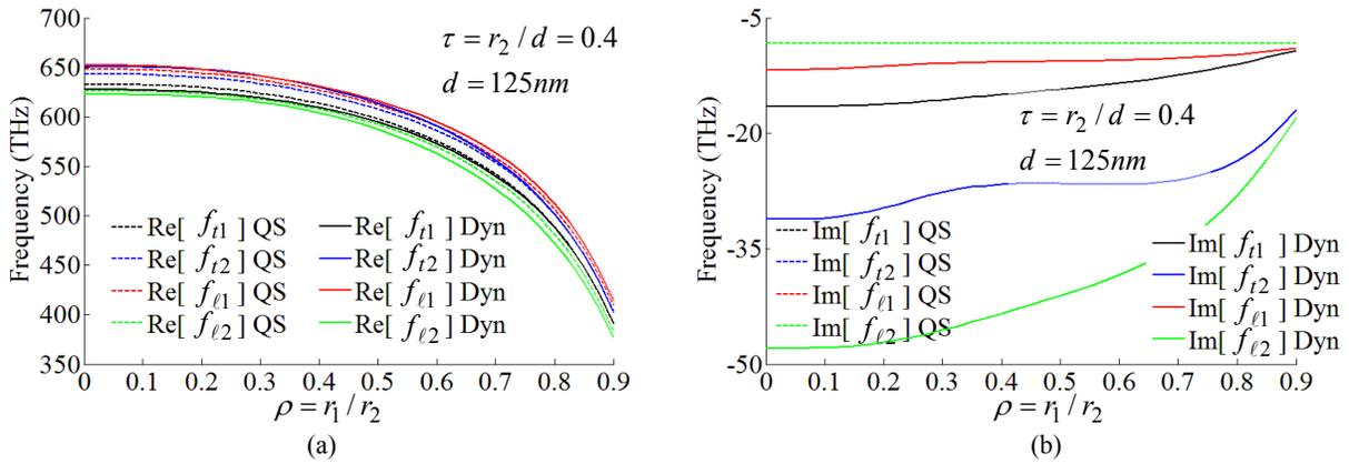
Fig. 5. Real and imaginary parts of the four resonance frequencies versus ratio of radii, for a sphere distance  $d = 125$  nm ( $r_2 = 50$  nm) for the dielectric core-gold shell structure.
