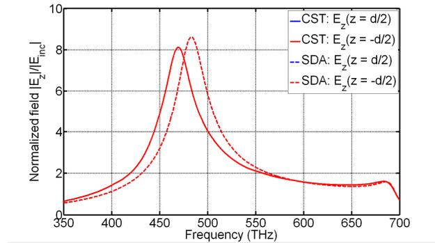
Fig. 14. Magnitude of the  $z$ -component of the electric field at the center of the shells, excited by a single plane wave arriving from the  $y$  direction, for the dielectric core-gold shell structure. Shell radius  $r_2=35$  nm, ratio of the radii  $\rho = r_1/r_2 = 0.8$  and center-to-center distance  $d=100$  nm.
