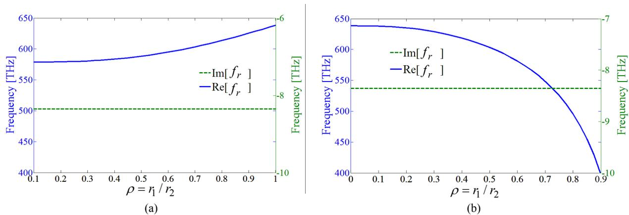
Fig. 3. Real and imaginary parts of the resonance frequency versus ratio of radii for a single nanoshell ( $r_2 = 50$  nm) for (a) the gold core-dielectric shell and (b) the dielectric core-gold shell structure.
