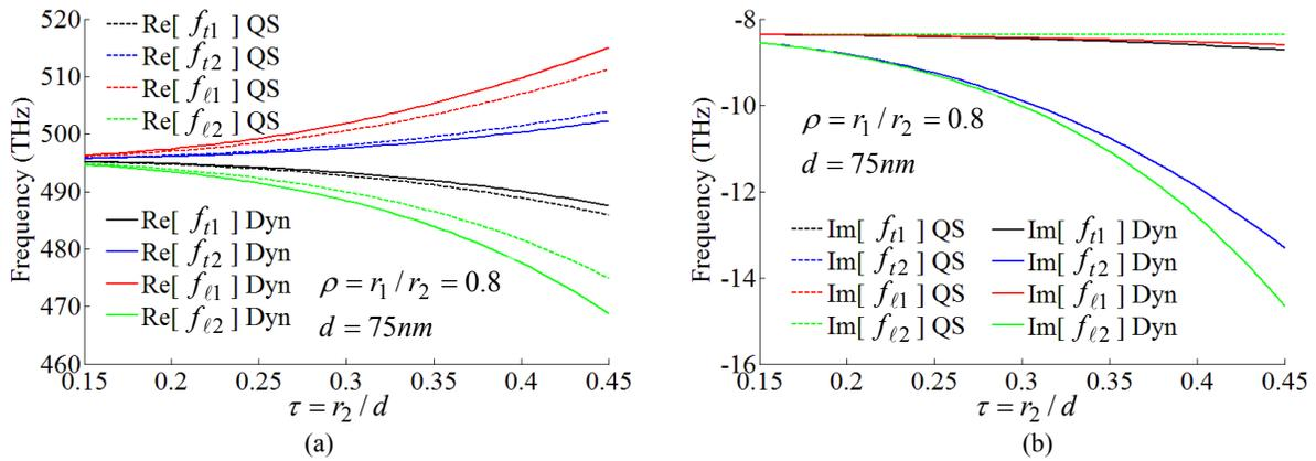
Fig. 7. Real and imaginary parts of the four resonance frequencies versus the ratio  $\tau = r_2/d$  for fixed distance  $d = 75 \text{ nm}$  between the nanoshells (i.e., the shell radius  $r_2$  is variable) and  $\rho = r_1/r_2 = 0.8$  for the dielectric core-gold shell structure.
