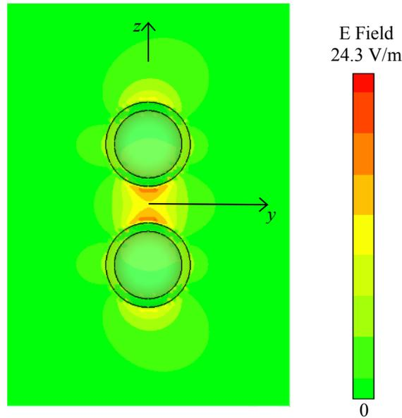
Fig. 16. Electric field distribution ( $z$ -component in the  $y$ - $z$  plane) for a pair of gold nanoshells (dielectric core and gold shell with  $r_2=35$  nm,  $\rho = r_1/r_2 = 0.8$ , and  $d=100$  nm) for the symmetric resonance mode excited by a single plane wave at  $f=469$  THz.
