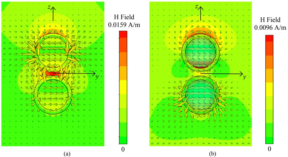
Fig. 13. As in Fig. 11 with the exception that now  $r_2=50$  nm and  $d=110$  nm. The antisymmetric and symmetric resonances (excited by a single plane wave) are shown at frequencies of  $f = 460$  THz and  $f = 485$  THz, respectively. Note that since the resonances are further apart the field at  $f = 460$  THz has a more clear antisymmetric field distribution than that in Fig. 11(a).
