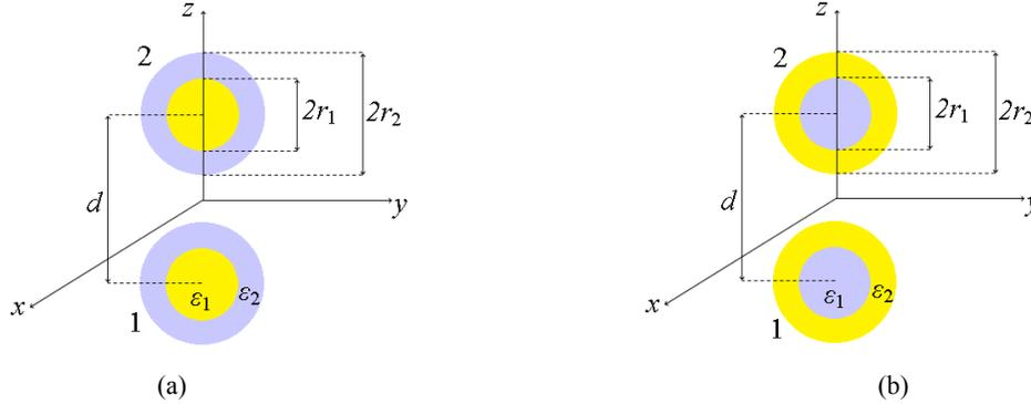
Fig. 1. Geometry of a pair of tightly coupled gold nanoshells. (a) Gold core and dielectric shell. (b) Dielectric core and gold shell.
