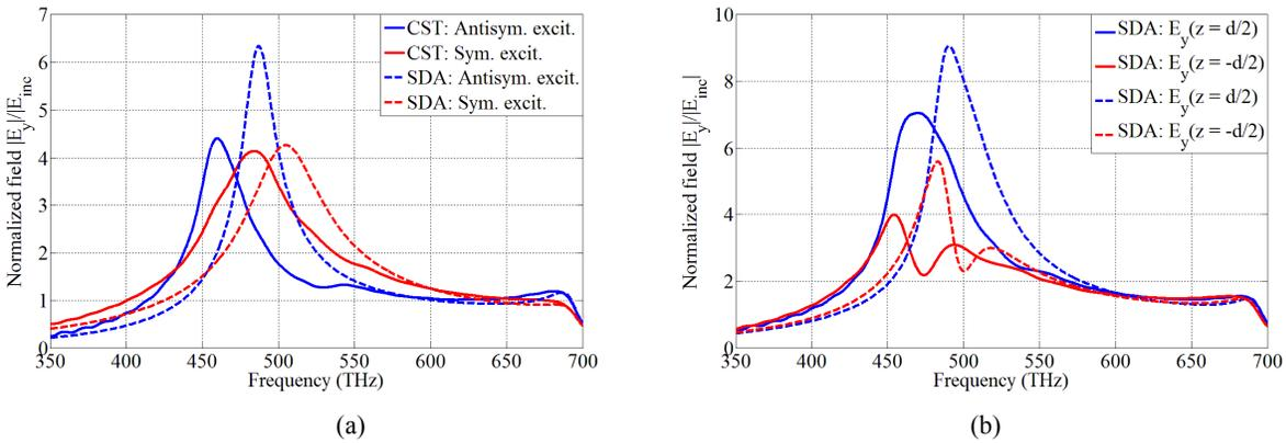
Fig. 12. As in Fig. 10, with the exception that now  $r_2=50$  nm and  $d=110$  nm. The main difference is that now the symmetric and antisymmetric resonances have a distance of 24.7 THz (further apart with respect to the case in Fig. 10).
