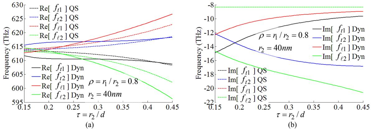
Fig. 8. Real and imaginary parts of the four resonance frequencies versus the ratio  $\tau = r_2/d$  for fixed shell radius  $r_2 = 40$  nm (i.e., the distance  $d$  between the nanoshells is variable) and  $\rho = r_1/r_2 = 0.8$  for the gold core-dielectric shell structure.
