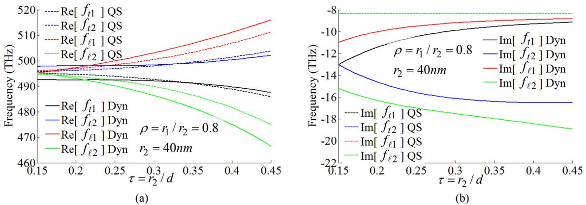
Fig. 9. Real and imaginary parts of the four resonance frequencies versus the ratio  $\tau = r_2/d$  for fixed shell radius  $r_2 = 40$  nm (i.e., the nanoshell distance  $d$  is variable) and  $\rho = r_1/r_2 = 0.8$  for the dielectric core-gold shell structure.
