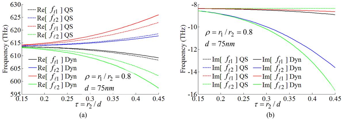
Fig. 6. Real and imaginary parts of the four resonance frequencies versus the ratio  $\tau = r_2/d$  for fixed distance  $d = 75 \text{ nm}$  between the nanoshells (i.e., the shell radius  $r_2$  is variable) and  $\rho = r_1/r_2 = 0.8$  for the gold core-dielectric shell structure.
