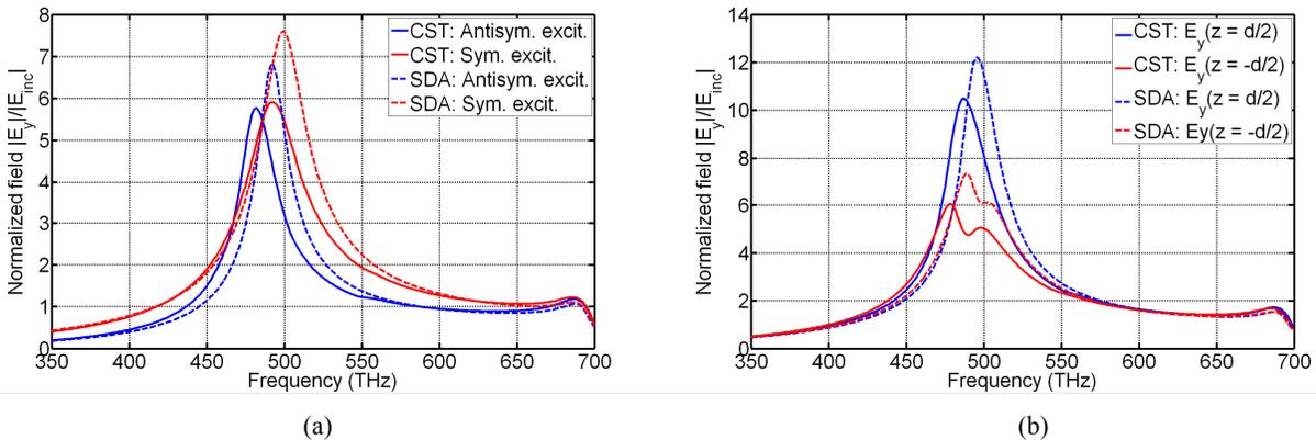
Fig. 10. Magnitude of the  $y$ -component of the electric field at the center of the nanoshells (dielectric core and gold shell with  $r_2=35$  nm, ratio of the radii  $\rho = r_1/r_2 = 0.8$  and center-to-center distance  $d = 100$  nm), excited by (a) a pair of antisymmetric or symmetric plane waves arriving from the  $+z$  and  $-z$  directions, and (b) a single plane wave coming from  $+z$ , for the dielectric core-gold shell structure.
