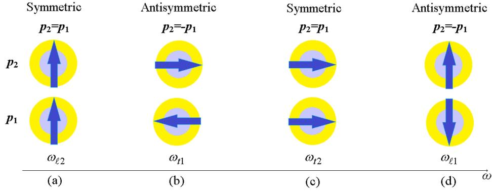
Fig. 2. Four possible resonance states in a pair of nanoshells. Both transverse ( $t$ ) and longitudinal ( $\ell$ ) resonance modes exhibit symmetric and antisymmetric configurations. The resonance order is the limiting case valid under the quasistatic (QS) approximation.
