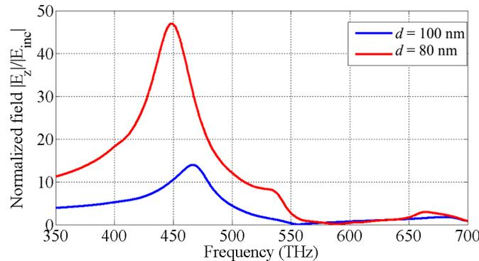
Fig. 15. Magnitude of the  $z$ -component of the electric field at the center of the pair system, excited by a single plane wave arriving from the  $y$  direction with electric field polarized along  $z$ , for the dielectric core-gold shell structure. Shell radius  $r_2=35$  nm,  $\rho = r_1/r_2 = 0.8$ , and center-to-center distance  $d=100$  nm and 80 nm. Note the amount of the strongest field enhancement in correspondence of the shortest  $d$ .
