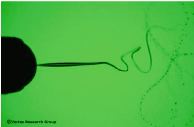
Fig. 6 Experimental profile of electrically charged droplet motion [18]
