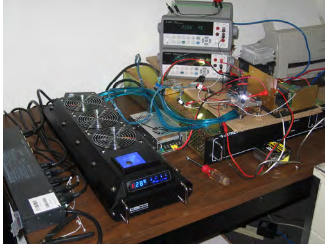
Figure 8.3: Experimental setup for measuring the thermal response of the LED.
