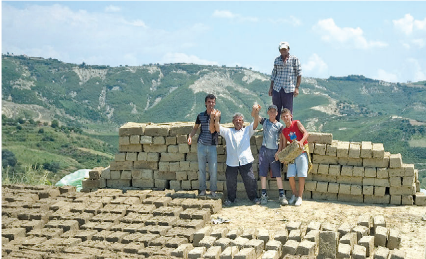
FIGURE 22.8 Dried mud bricks piled up, together with bricks at various stages of drying (in foreground)
