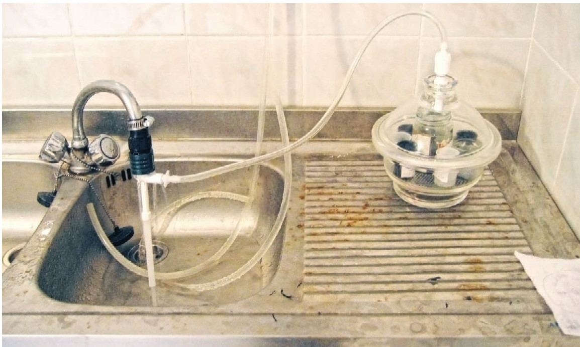
FIGURE 5.5 Treatment of copper alloy artifacts with BTA under vacuum using a small glass desiccator and running water from the sink faucet to draw a vacuum
