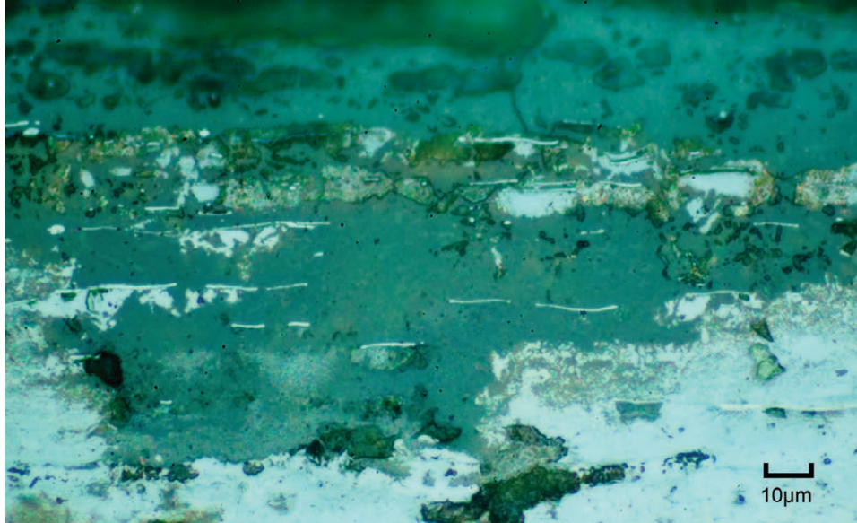
FIGURE 11.7 The light-colored inclusions within the sample taken from 10/59 (SF 336) appear flattened due to the hammering used to create the flat pendant. Other objects sampled from Lofkënd, such as 10/31 (SF 227), 10/61 (SF 163a–d), and 10/78 (SF 163h), also have inclusions that appear flattened due to cold working that took place during manufacture.
