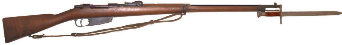
FIGURE A3.5 Mannlicher-Carcano M 1891, 6.5-mm caliber rifle produced from 1892 to 1945 and used by Italian troops during World War I and War World II
