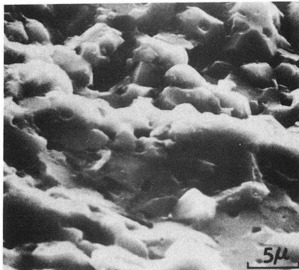
Fig. 39. Scanning electron fractograph of the undoped MgO compact sintered at 1430°C for 730 min in static air atmosphere; P = 0.10 .
