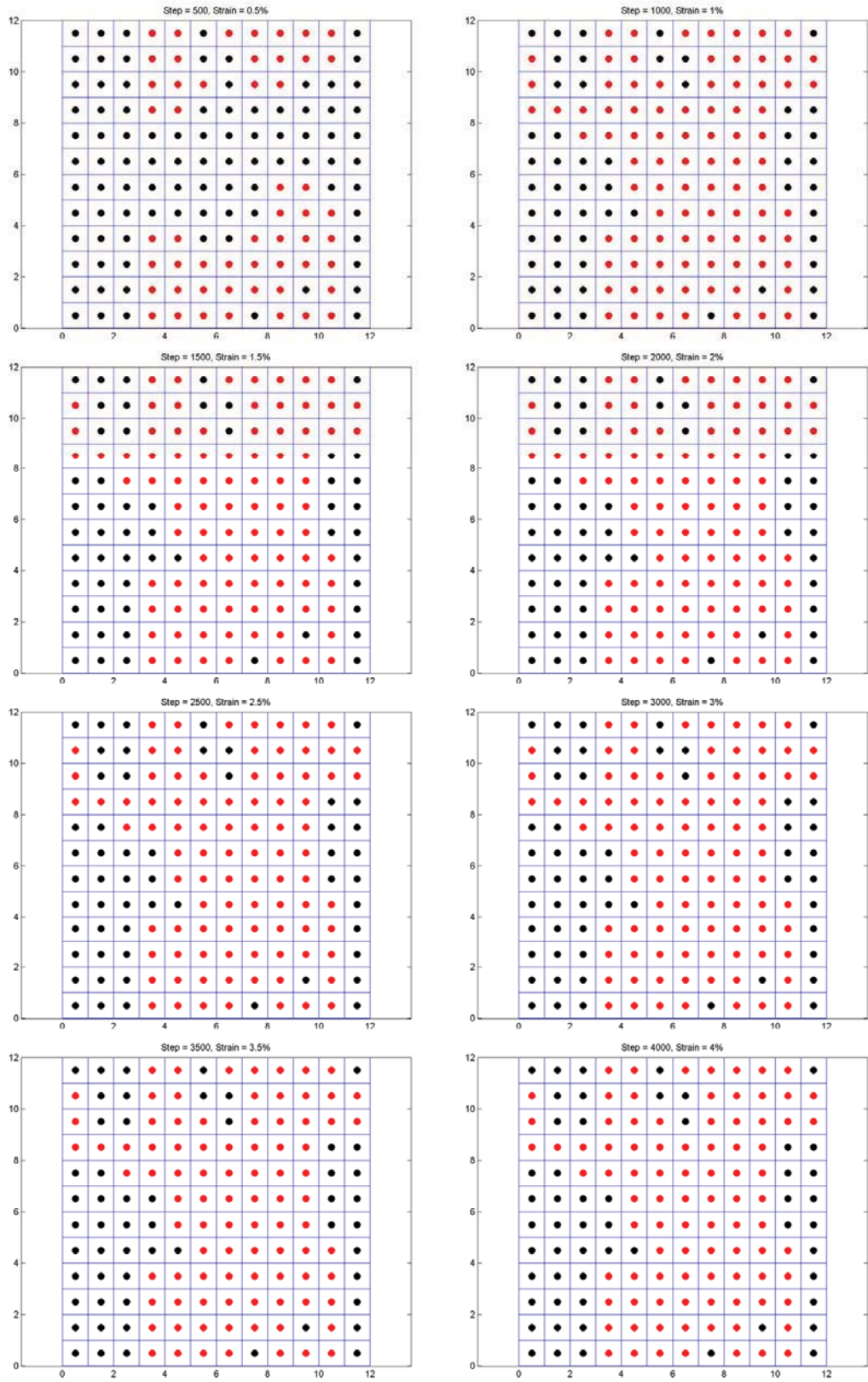
Figure 4.26 Damage evolution of broken fibers in the composite – Mechanism 3
