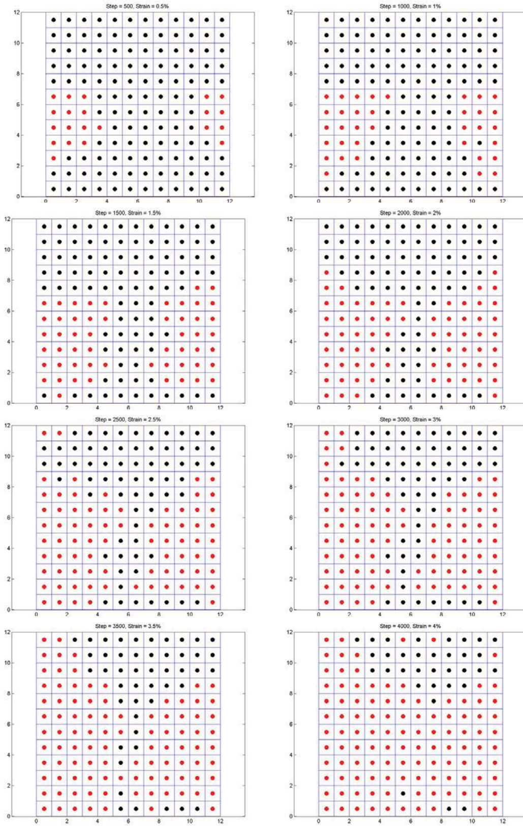
Figure 4.27 Damage evolution of broken fibers in the composite – Mechanism 4
