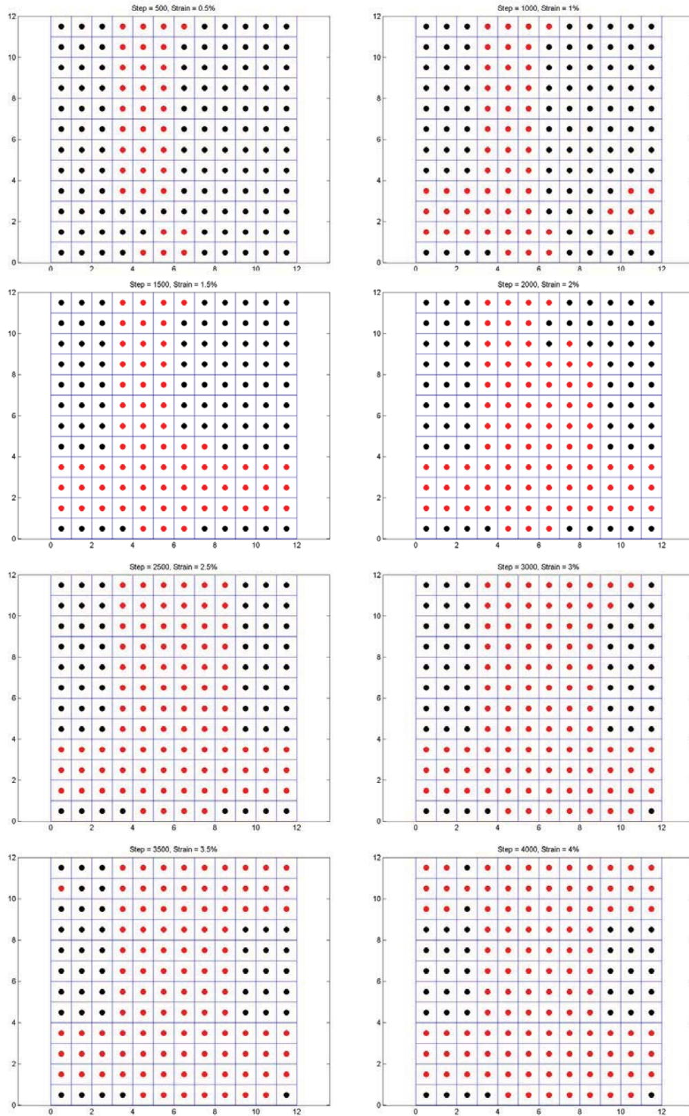
Figure 4.24 Damage evolution of broken fibers in the composite – Mechanism 1
