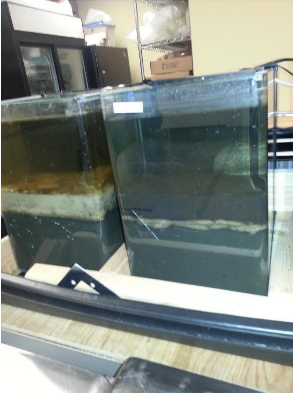
Dark top layer is the amendment zone, white layer is a quartz layer, and dark lower layer is the homogenized sediment. The total height of the solids shown is 20 cm.
