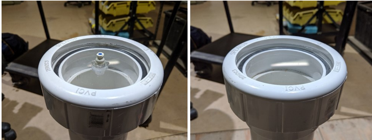
Figure 6. PAWS housing with PVC union threaded endcaps and collars. The front and rear doors (left and right respectively) are made from laser cut clear acrylic. The pass through in the front door is an IV valve epoxied into a laser cut, or drilled, hole through the center of the disc.
