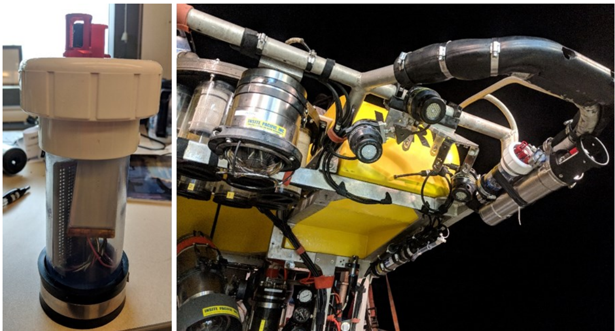
Figure 9. Pressure and temperature logger built with the same general architecture as PAWS sitting on the bench (left). Both the logger and PAWS use an Adafruit M0 express microcontroller. The logger uses temperature and pressure sensors from Blue Robotics. This version of the logger was built in a 2-inch PVC housing with a PVC union and laser cut acrylic door on one end, and a rubber cap on the other. We tested the logger down to 1000m alongside a commercial CTD package on the ROV Hercules . To handle the high pressures, the housing was filled with mineral oil and the rubber cap acts as pressure compensator. Future versions of PAWS will incorporate sensors for parallel data logging, or to act as a sampling trigger.
