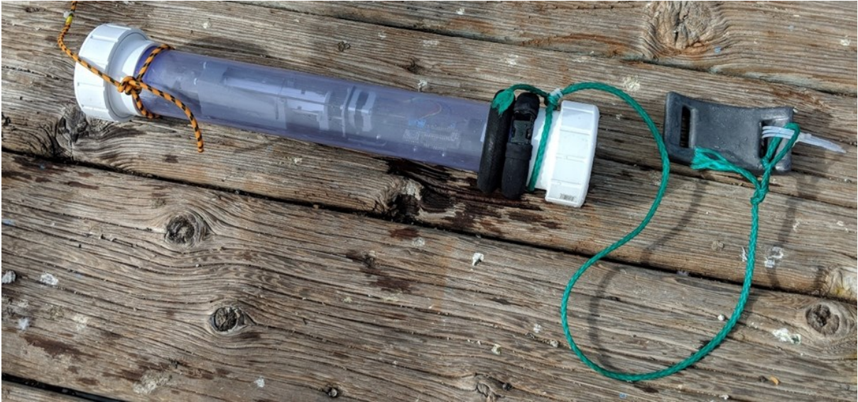
Figure 1. PAWS on a pier ready for deployment. The black bands are SCUBA diving ankle weights. The dive weight attached to the green rope hits the seafloor before the sampler does allowing PAWS to be anchored above the bottom reducing the possibility of particulate matter blocking the sampler's inlet.
