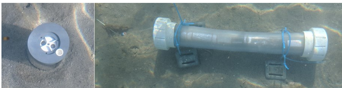
Figure 8. Benthic flux chamber (left) and PAWS (right) deployed at 1m water depth in Mo'orea, French Polynesia. The flux chamber consists of a 10cm clear tube capped with a sealed lid (grey) which contains a manual magnetic stir propellor (center white) and a rubber septum for sampler collection with a syringe (edge white). The chamber is driven into the seafloor to collect potential chemical fluxes over a 12-hour period. The PAWS system was deployed alongside three flux chambers to collect a comparison sample of ambient seawater.
