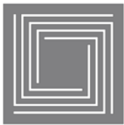
Figure 1: Top view of multi-turn beam structure
