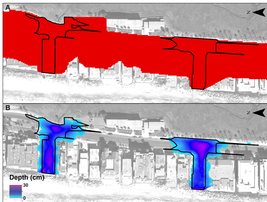
Figure 2. (A) A static flood prediction; and (B) a hydrodynamic flood prediction using XBeach nonhydrostatic as an overtopping model along with field validation data (black outline). Note depth is unavailable in static predictions and is shown only as extent in red.
