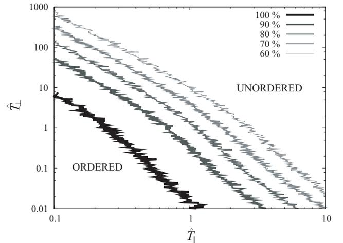
FIG. 2: Reflection probability map numerically obtained from the universal Hamiltonian (14). We have considered a round beam where  $\hat{T}_x = \hat{T}_y$ . The initial value of the longitudinal coordinate  $\hat{z}$  has been fixed at 100, which is not essential to the result; even if a different value is chosen, we eventually find almost the same map as long as it is sufficiently larger than 10.
