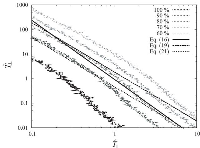
FIG. 5: Reflection probability map. The dotted curves are the probability contours shown in Fig. 2. The thick broken and dotted lines indicate the reflection borders given, respectively, by Eq. (19) and (21). The phenomenological fit of Eq. (16) has also been plotted in a thick solid line.
