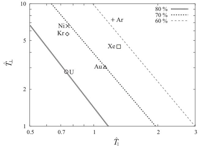
FIG. 3: The operating points at which the anomalous beam behaviors were observed in ESR have been marked with + ( $^{40}\text{Ar}^{18+}$ ),  $\times$  ( $^{58}\text{Ni}^{28+}$ ),  $\diamond$  ( $^{86}\text{Kr}^{36+}$ ),  $\square$  ( $^{132}\text{Xe}^{54+}$ ),  $\triangle$  ( $^{197}\text{Au}^{79+}$ ), and  $\circ$  ( $^{238}\text{U}^{92+}$ ). The data used here have been summarized in Table I. The three lines show the smoothed probability contours in Fig. 2
