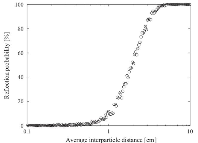
FIG. 6: Two-particle simulation result corresponding to an ESR experiment. A 360 MeV/u  $^{197}\text{Au}^{79+}$  beam in ESR with  $\nu_0 = 2.3$  have been assumed. Unlike the numerical procedure outlined in Sec. IV, the initial value of  $|\hat{p}_z|$  has been fixed at  $\sqrt{\hat{T}_\parallel}$  in each simulation.
