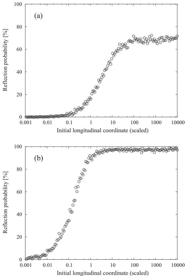
FIG. 1: Dependence of reflection probability on the initial value of  $|\hat{z}|$ . The initial conditions assumed in these examples are: (a)  $\hat{T}_\perp = 50, \hat{T}_\parallel = 0.3$ ; (b)  $\hat{T}_\perp = 0.1, \hat{T}_\parallel = 0.7$ .
