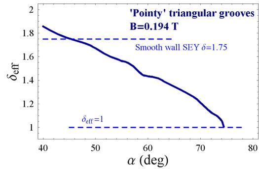
Figure 3: Effective SEY as a function of the steepness angle  $\alpha$  as derived from the simulation of e-cloud build-up.
