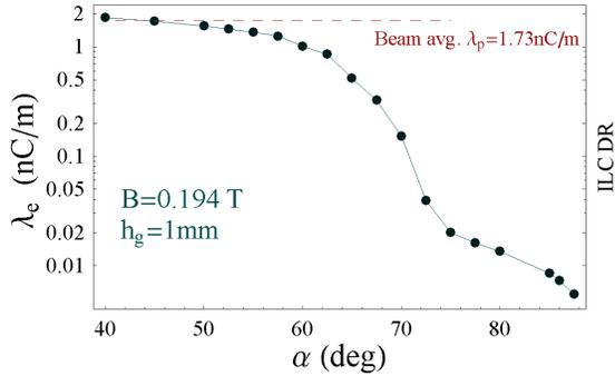
Figure 2: Maximum linear density of electrons accumulated during a passage of a train of positron bunches in a ILC damping ring dipole vs. steepness angle  $\alpha$  of triangular grooves (with sharp edges). Al chamber with  $\delta_{\max} = 1.75$ .
