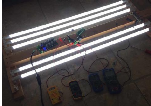
Figure 37: Direct-DC Zone Light Prototype
