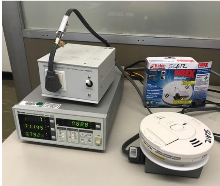
Figure 50: Power Measurement Test Configuration
