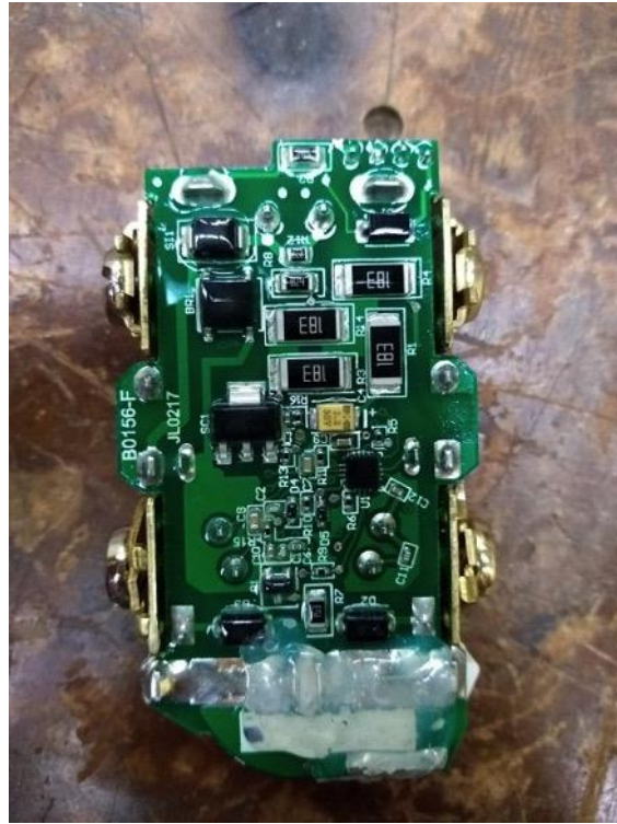
Figure 59: GFO17 GFCI Outlet Teardown—Electrical Circuit
