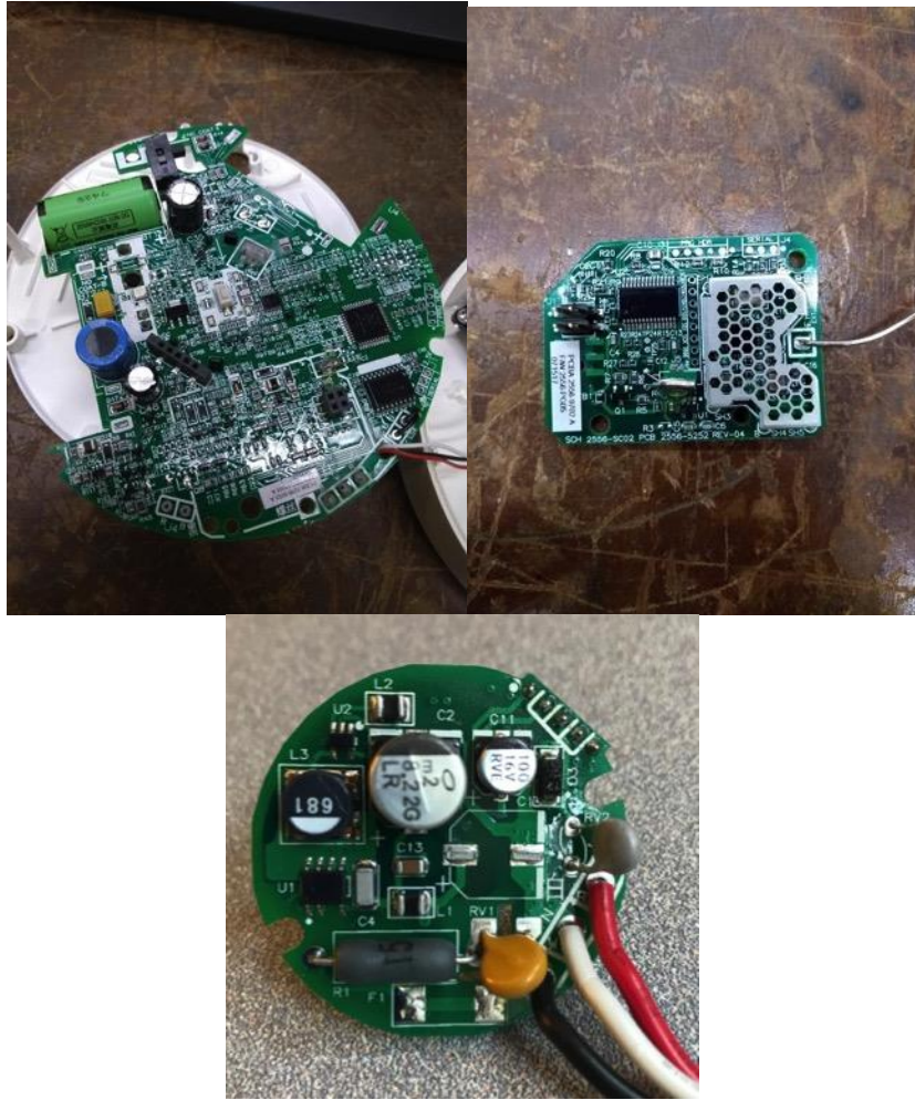
From top left clockwise: main PCB, power PCB, and wireless PCB.
