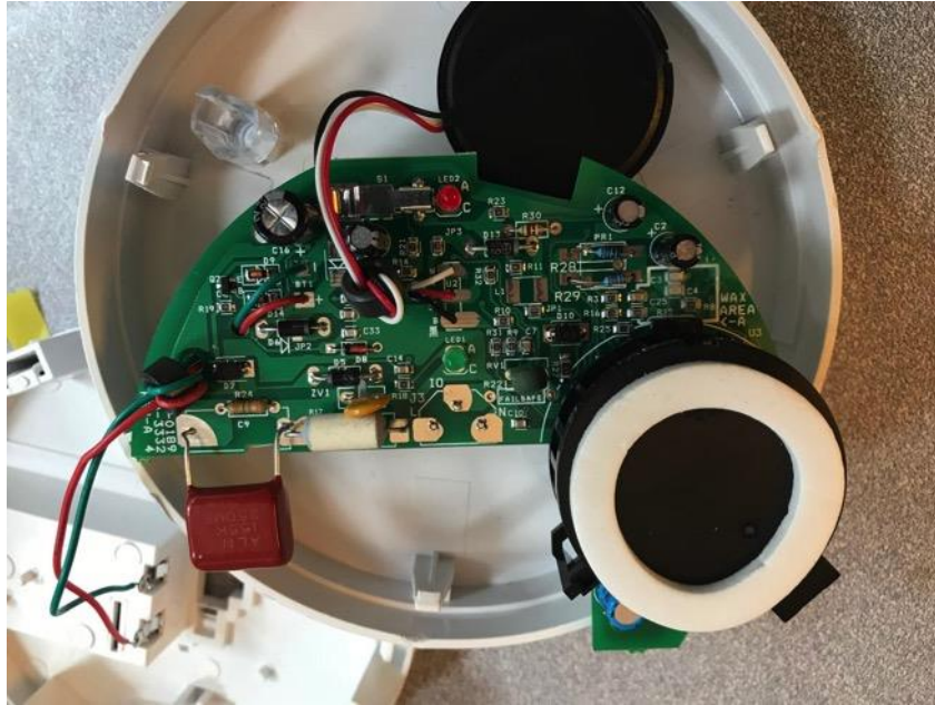
Figure 60: Teardown of the SMA36 Smoke Alarm—Electric Circuit
