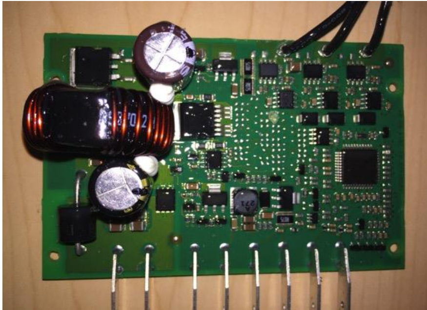
Figure 32: Danfoss/Secop Inverter Board
