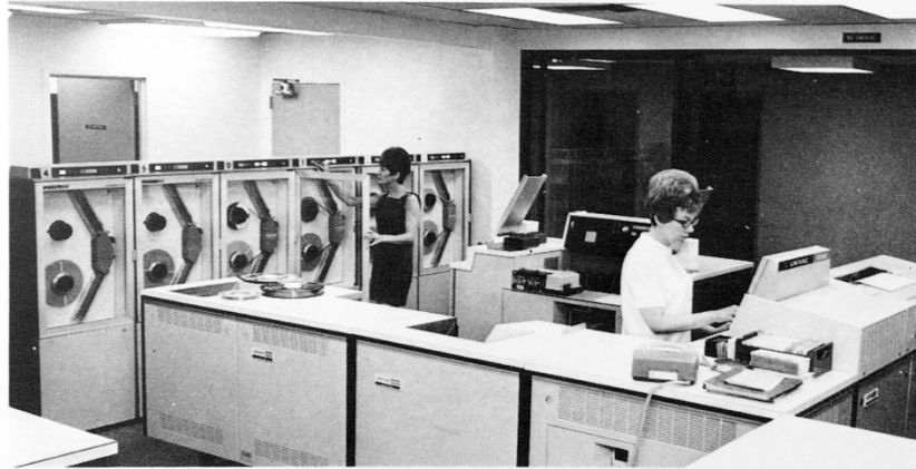
Computer Services Center—On command, DMJM's Univac 9300 Data Communication System can be pulsed with any one of three Univac 1108 systems, the DMJM installation performing input/output functions and the 1108 providing its computation and storage capabilities. As required by workload, a Univac Data Communication Terminal 2000 is being phased into each regional office operation, giving that office ready access either to the Los Angeles 9300 system or to the nearest 1108 system.
