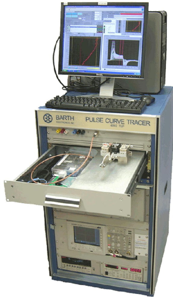
Fig. 1.4 A BARTH Model 4002 TLP tester used in the testing.
