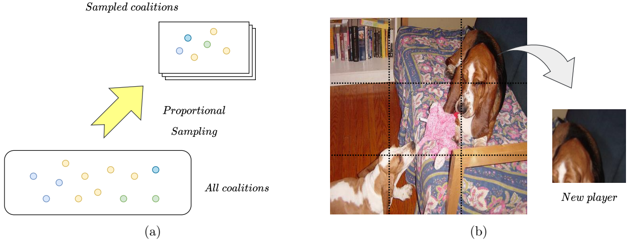
Figure 2.2: (a) Proportional sampling in our SIG. Different colored nodes represent different weights defined by Equation 2.9. (b) Construction of new players. A patch of pixels is considered a new player/feature on which we search the baseline set.
