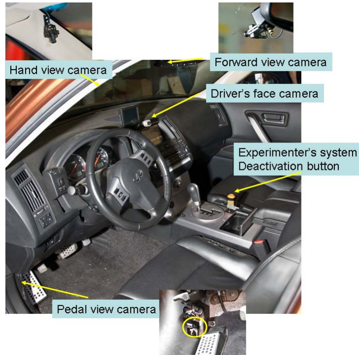
Figure 32: Vehicle Interior, Showing Locations of Video Cameras
