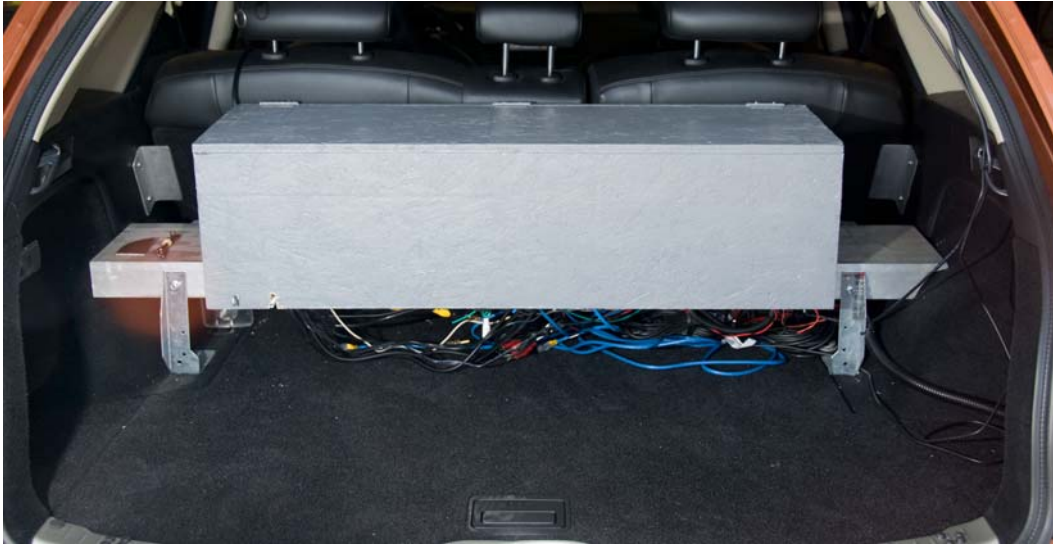
Figure 30: Computer enclosure in luggage compartment behind rear seat of vehicle, with cover closed
