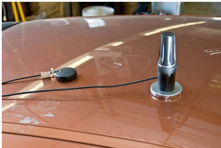
Figure 31: DGPS Antenna (left) and DSRC Communication Antenna (right)
