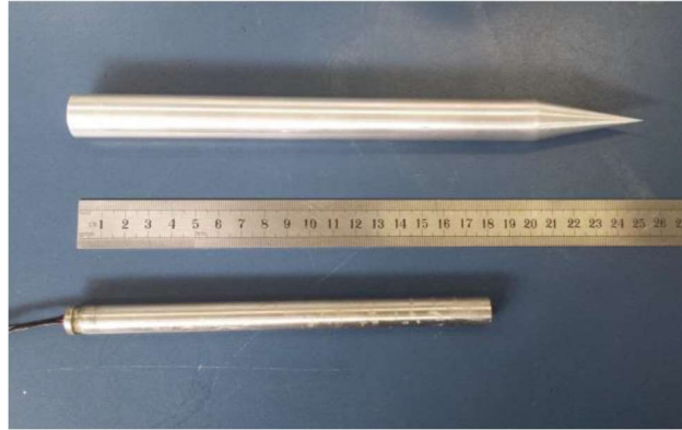
Figure2. Torpedo pile and heating element
