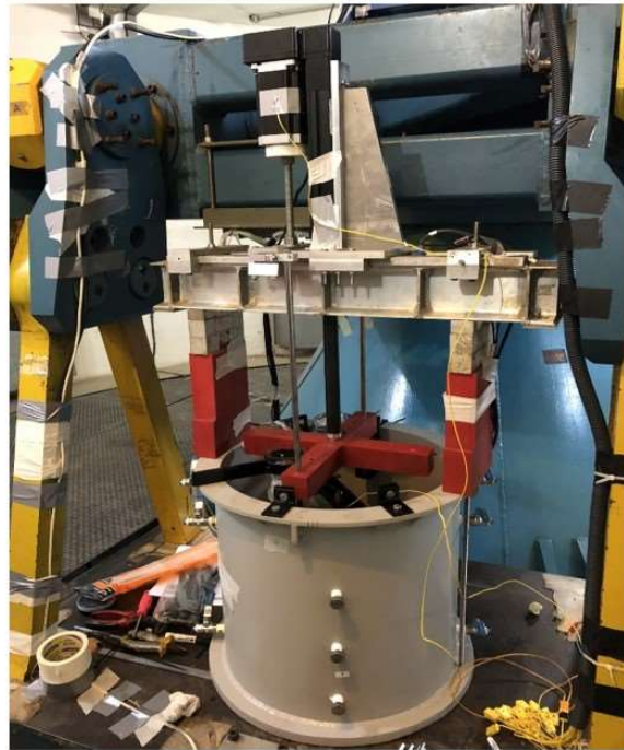
Figure 4. T-bar support structure and positioning of the T-bars and their installation in the centrifuge.
