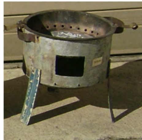
Fig. 4. Mirak stove: height: 32 cm; diameter: 30.5 cm; weight: 2.8 kg.
