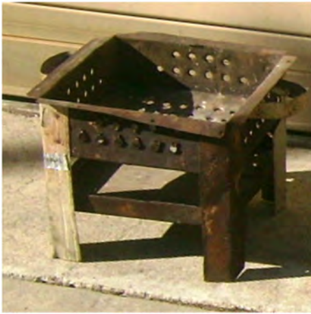
Fig. 1. Traditional Haitian stove: height: 27 cm; length/width: 11 cm; weight: 2.8 kg.
