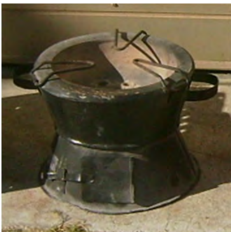
Fig. 2. EcoRecho stove: height: 22 cm; diameter: 27.5 cm; weight: 6.2 kg.
