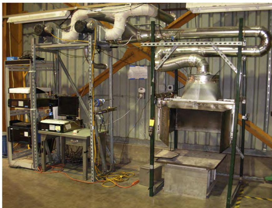
Fig. 5. The stove testing system at LBNL. The exhaust hood and ductwork is seen on the right-hand portion of the photo; the instrumentation is on the left.
