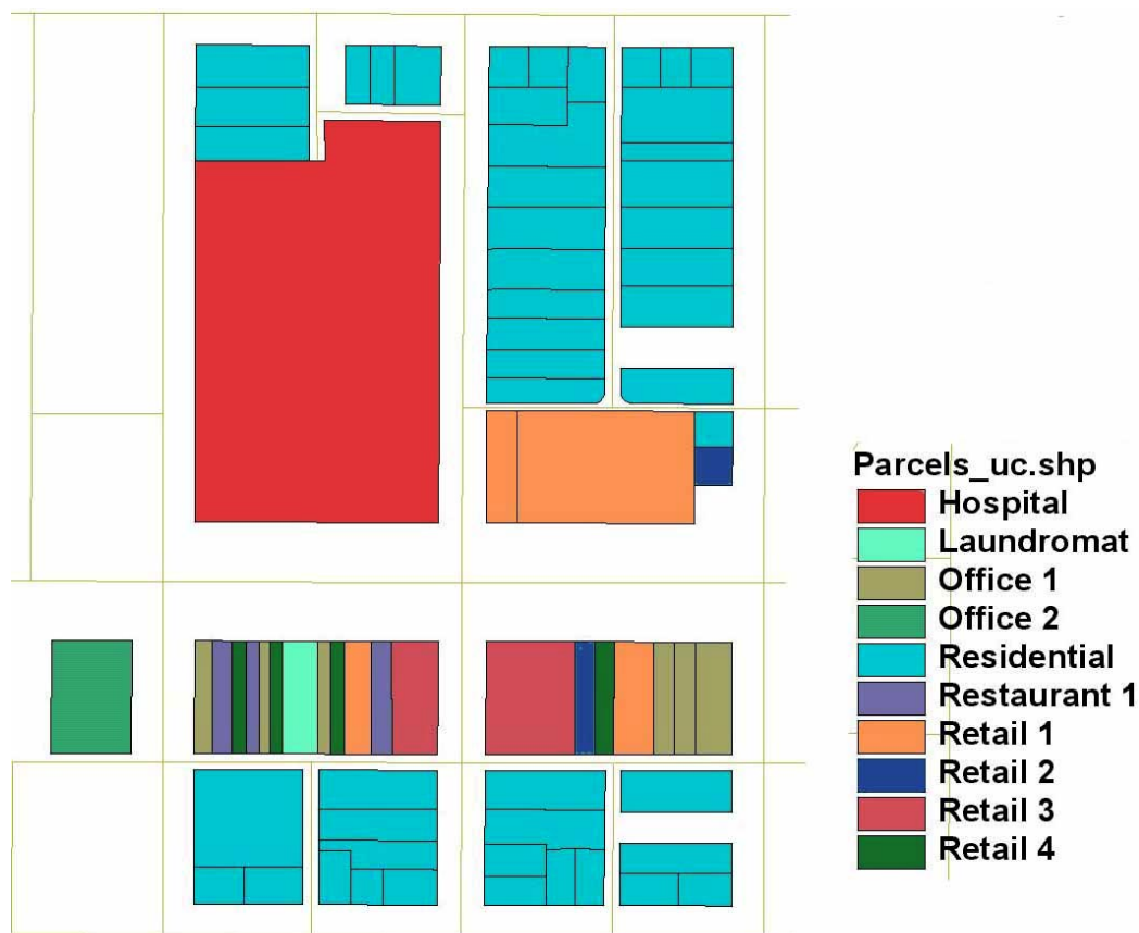
Figure 10. GIS map of individual buildings, classified according to their energy needs. For more detail on each of the building classifications, see Appendix B on load-shape preparation.
