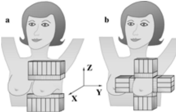
Figure 1. The most common PEM camera geometry is the parallel plane geometry shown in a). A variant rectangular geometry is shown in b).
