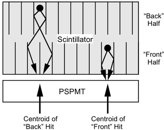
Figure 3. A method for determining the depth of interaction. Interactions that occur in the “front” section of the scintillator produce light whose centroid (at the PSPMT entrance) is at the center of the scintillator pixel. Interactions that occur in the “back” section of the scintillator block produce light whose centroid is at the edge of the scintillator pixel (*i.e.*, offset by half of a crystal width).
