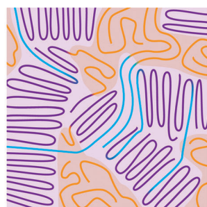
Initial undoped film with good morphology and lots of tie chains (blue lines)
