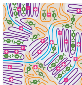
Sequential doping from CB allows \text{F4TCNQ} to infiltrate crystalline domains, increasing doping level but reducing doping efficiency, reducing conductivity
